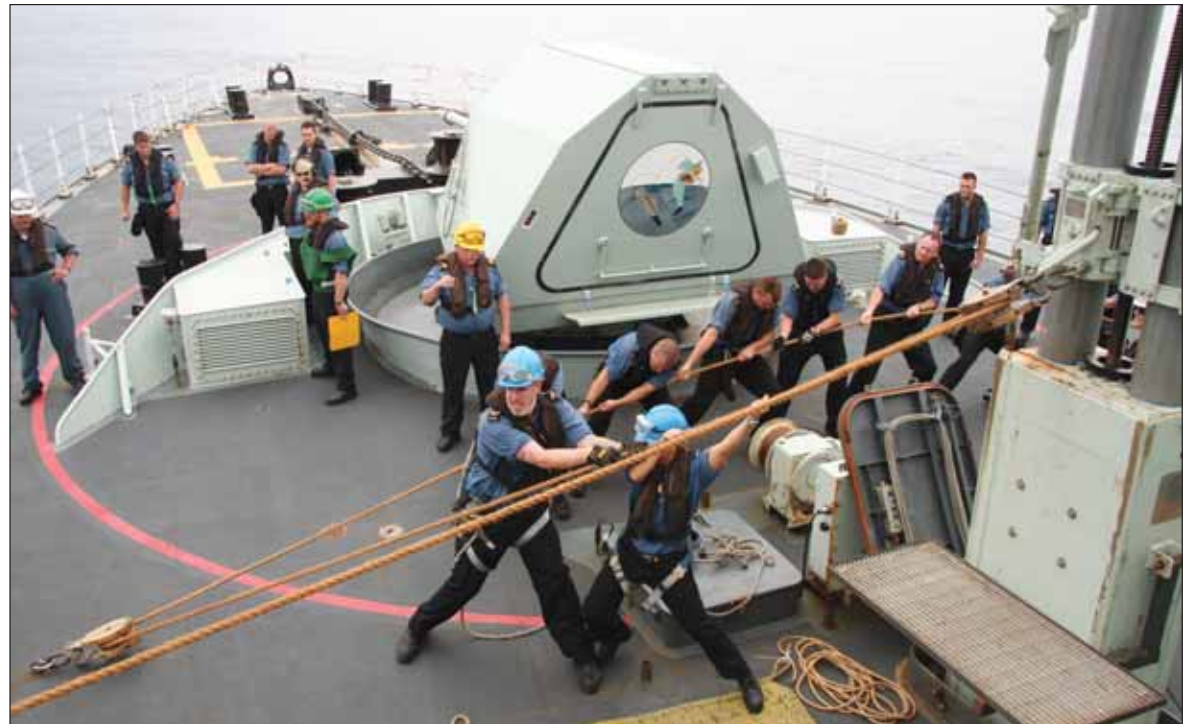
The deck department on board HMC Regina works tirelessly to pull over the line for a heavy jackstay in the waters off Hawaii. This is the method used at sea to transfer heavy goods.
