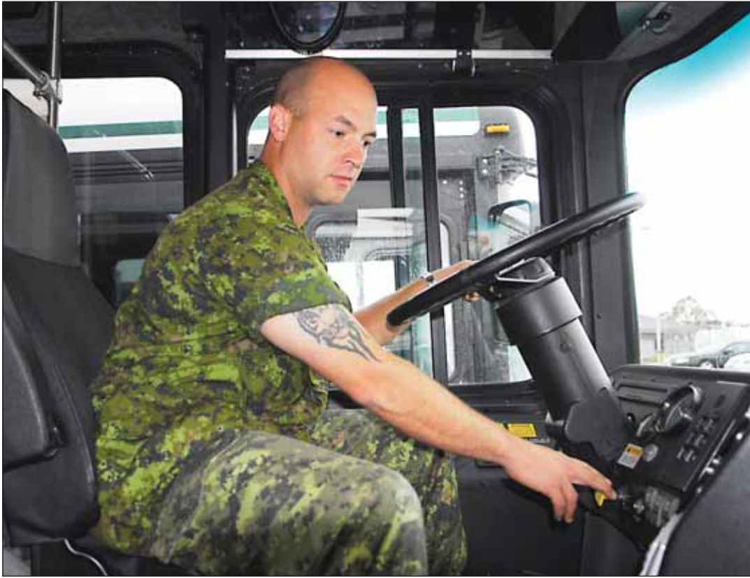
Above: Cpl Dallas McKeough, mobile support equipment operator, tests the air brakes on a Thomas 38 passenger bus as part of a safety inspection transport employees perform regularly.
