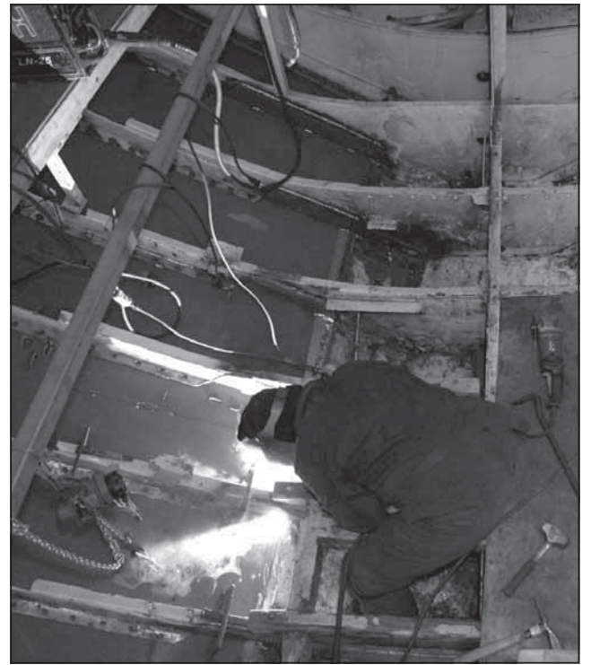
Shelley Lipke, Lookout Welder Derek Lintaman works on HMCS Oriole , welding steel to replace the 88-year-old hull. The ship is being worked on at Point Hope Shipyard and is due to return to the navy Feb. 27.
