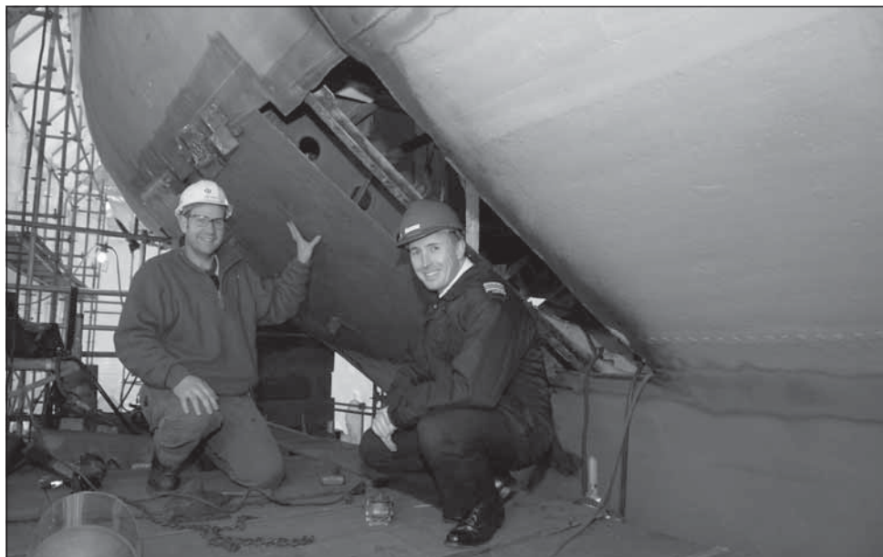
Shelley Lipke, Lookout Welder Derek Lintaman works on HMCS Oriole , welding steel to replace the 88-year-old hull. The ship is being worked on at Point Hope Shipyard and is due to return to the navy Feb. 27.
