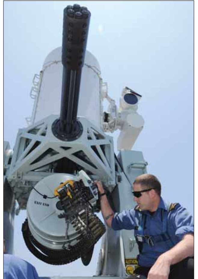
LS Randy Melancon cycles live rounds through the Close-in Weapon System in order to replace them with dummy rounds for maintenance following a live fire exercise.
