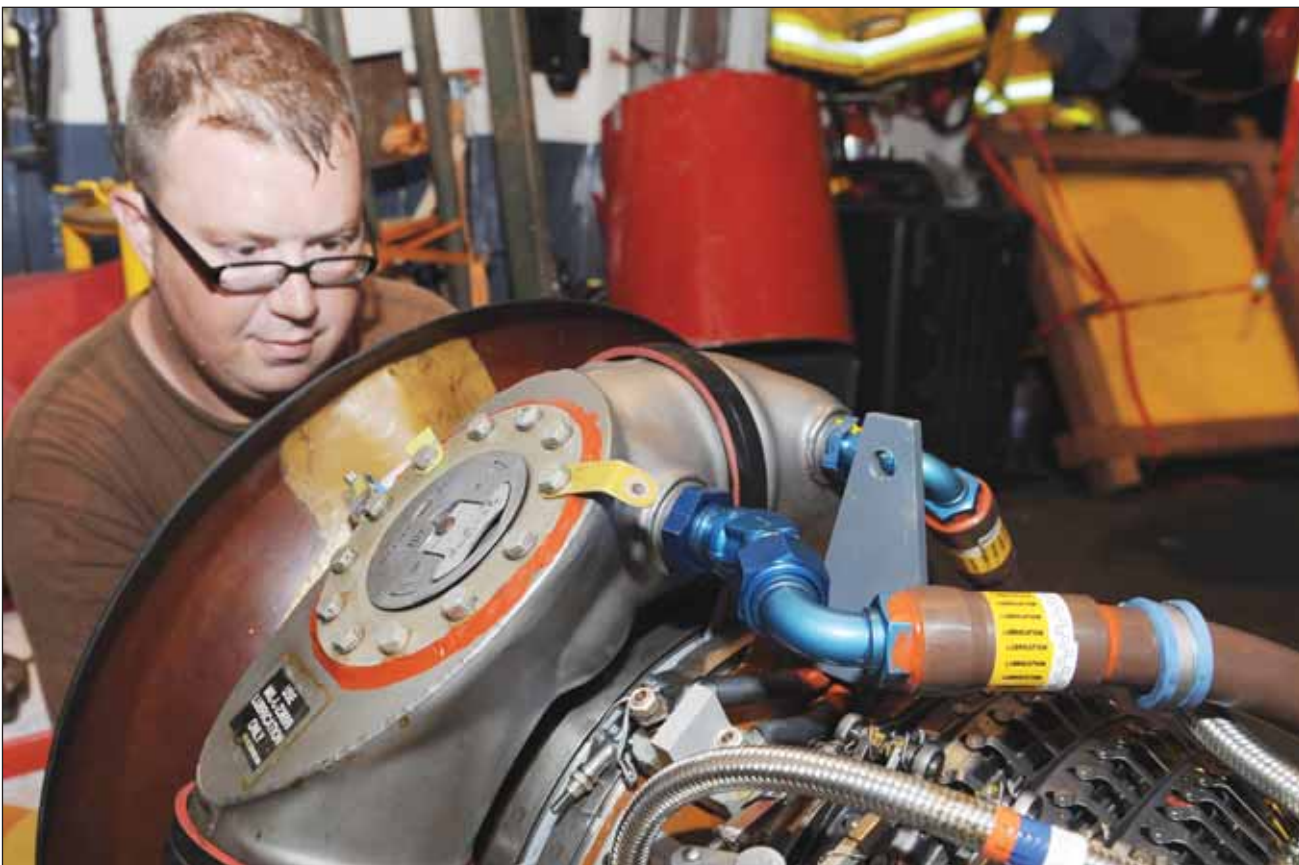
Cpl Dave Redecopp, an aviation system technician, prepares a replacement engine for the CH 124 Sea King helicopter on board Winnipeg.
