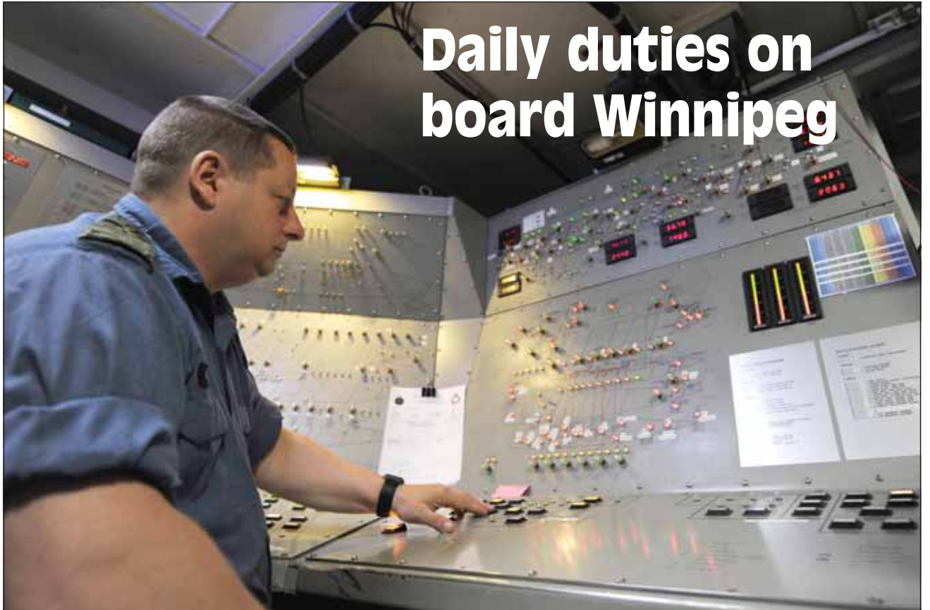
Above: Sgt Guy Croteau, a resource management services clerk, monitors the damage control console in HMCS Winnipeg's machinery control room. As part of his secondary duties, Sgt Croteau watches for potential alarms that notify if there is a fire or flood in the ship.
