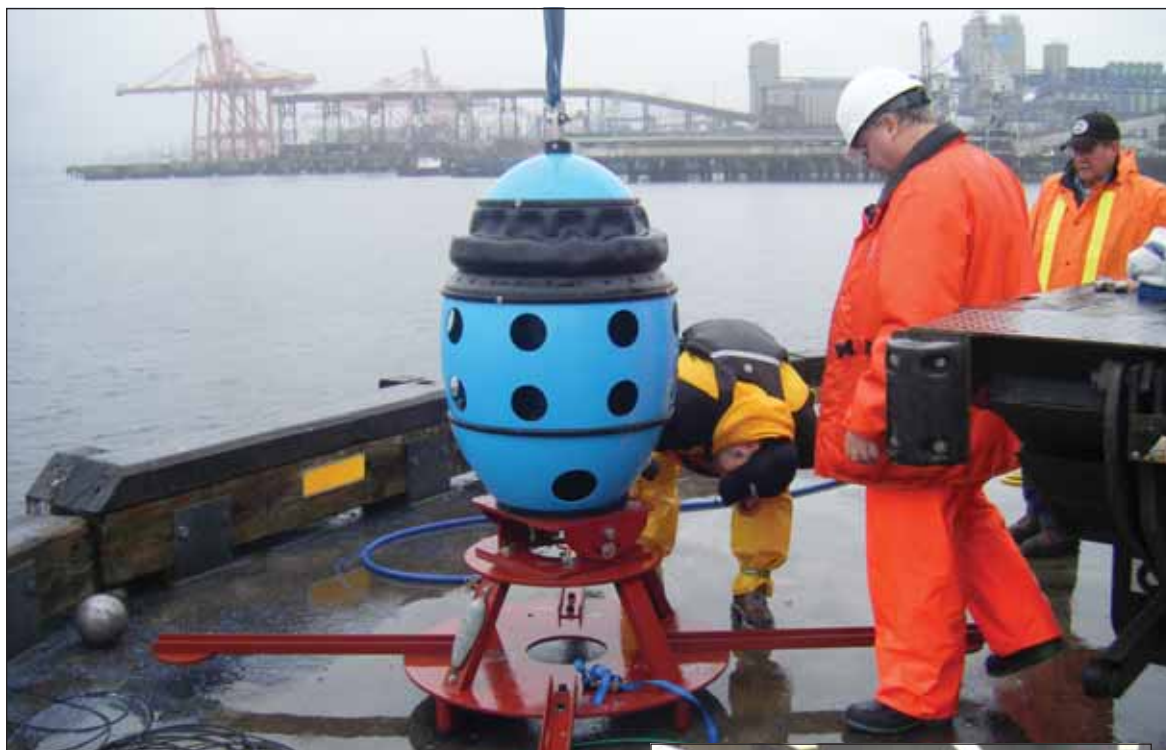
Above: Crane operators and scientists prepare to submerge an underwater sonar system to the ocean floor of Vancouver Harbour for diver detection trials. Ten members from Fleet Diving Unit Pacific dove toward the system to see how quickly it tracked them.
