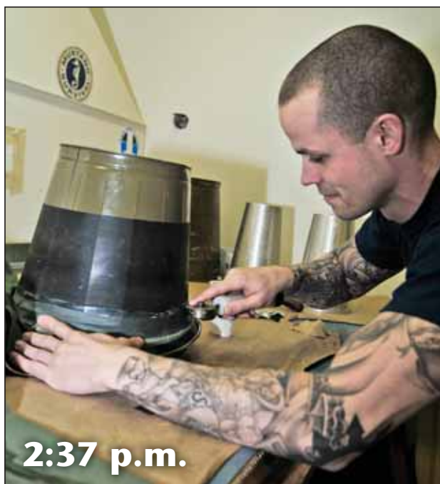
Left: Cpl Matthew Cumming glues a seal on a waterproof flying suit to ensure it's 100 per cent waterproof. Keeping the equipment in good condition is a big job at 443, and the safety of the crew and passengers depends on life rafts, vests and suits being waterproof and safe.
