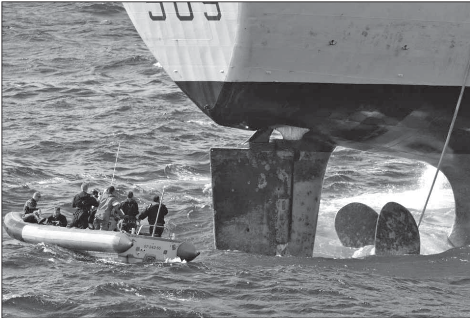
Cpl Charles A. Stephen, MARPAC Imaging HMCS Protecteur's dive team assesses the extent of the damage to the ship's propeller after a tow rope got wrapped around the propeller during a tow exercise in September. Fleet Maintenance Facility Cape Breton has found an innovative way to repair the propeller.
