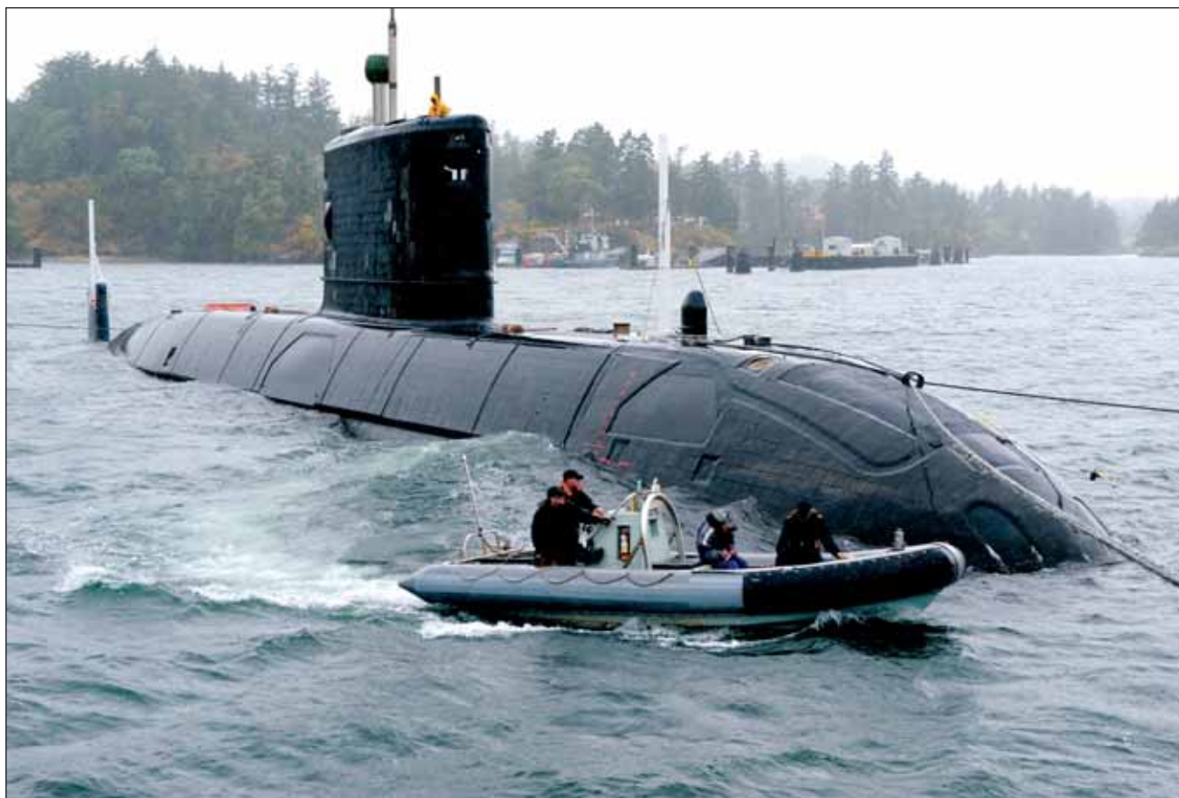
HMCS Victoria conducted a series of static dives as part of post-refit trials. The controlled dives were done in the harbour to allow submerged testing of various systems.
