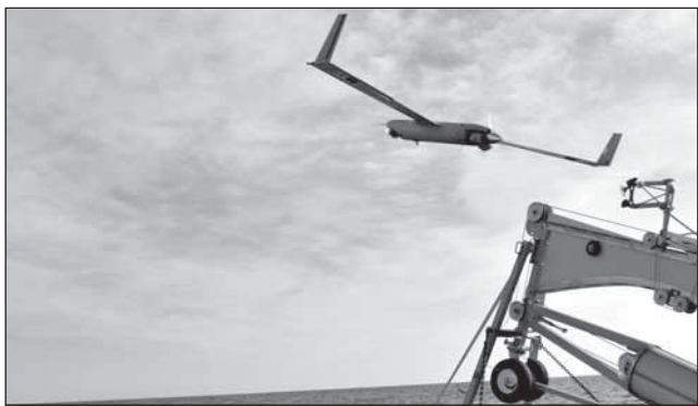
Above: Garth Matheson (left), a field service representative, observes Pat Brophy, Director UAV Services, operating the support legs of the recovery system for the UAV in order to secure it to the flight deck.
