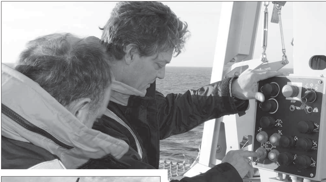
Above: Garth Matheson (left), a field service representative, observes Pat Brophy, Director UAV Services, operating the support legs of the recovery system for the UAV in order to secure it to the flight deck.
