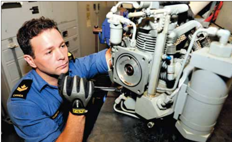
Photo by Cpl Ronnie Kinnie, Formation Imaging Services MS Stephen Hawco, weapons engineering technician onboard HMCS Charlottetown, conducts maintenance on a Close in Weapons System compressor motor while in the Red Sea on Operation Metric.
