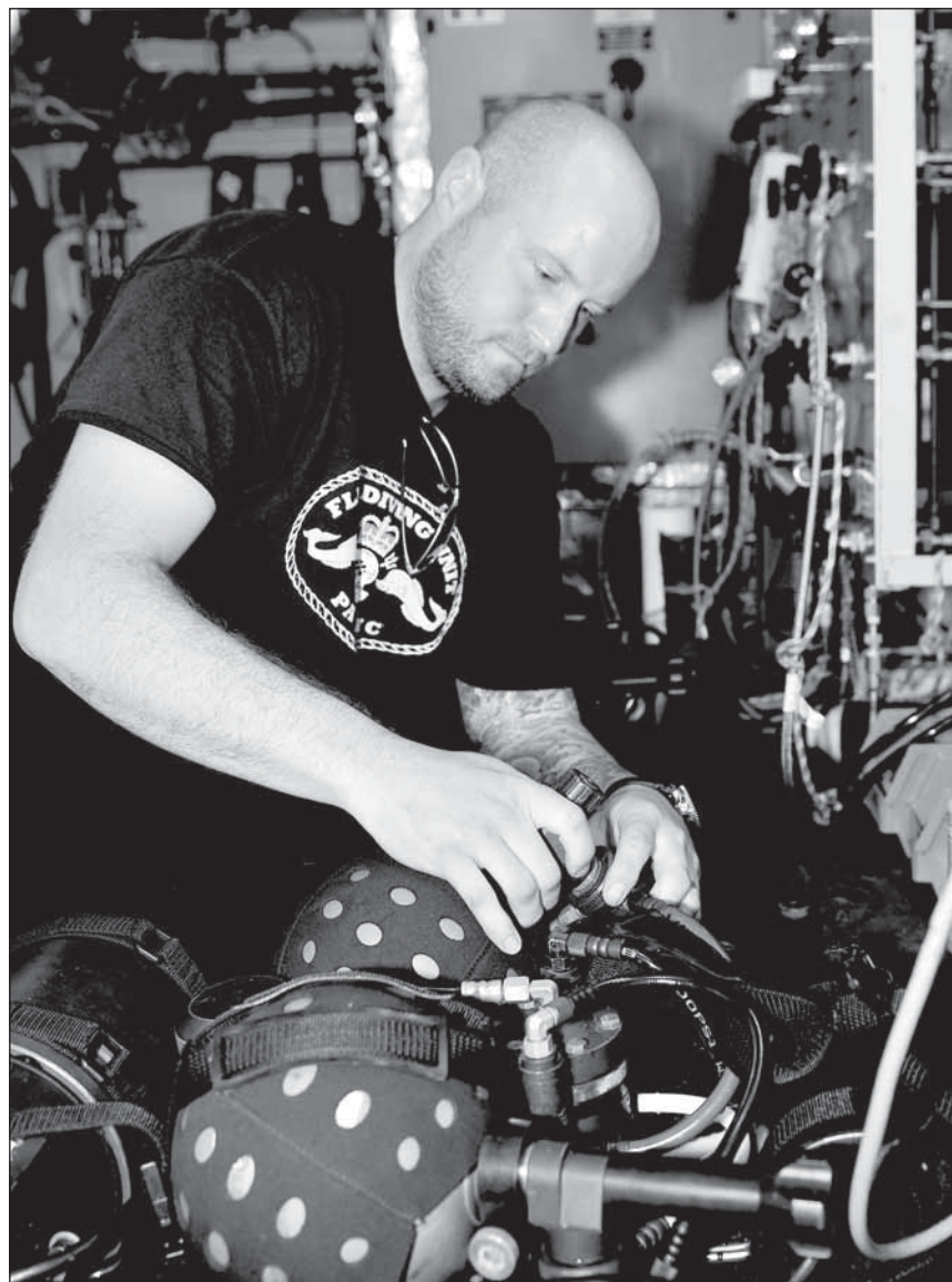
Photos by Shelley Lipke, Lookout Standby clearance diver and Canadian Underwater Mine Apparatus technician LS Adam King fixes a regulator on the rebreather on board YDT II.
