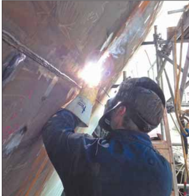
A welder repairs part of the hull on HMCS Winnipeg.
