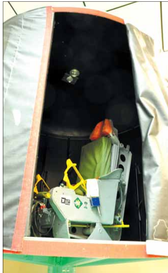
A CF-101 Voodoo fighter aircraft ejection seat is bolted to the inside of a spinning, tilting chamber that is used to desensitize people to air sickness.
