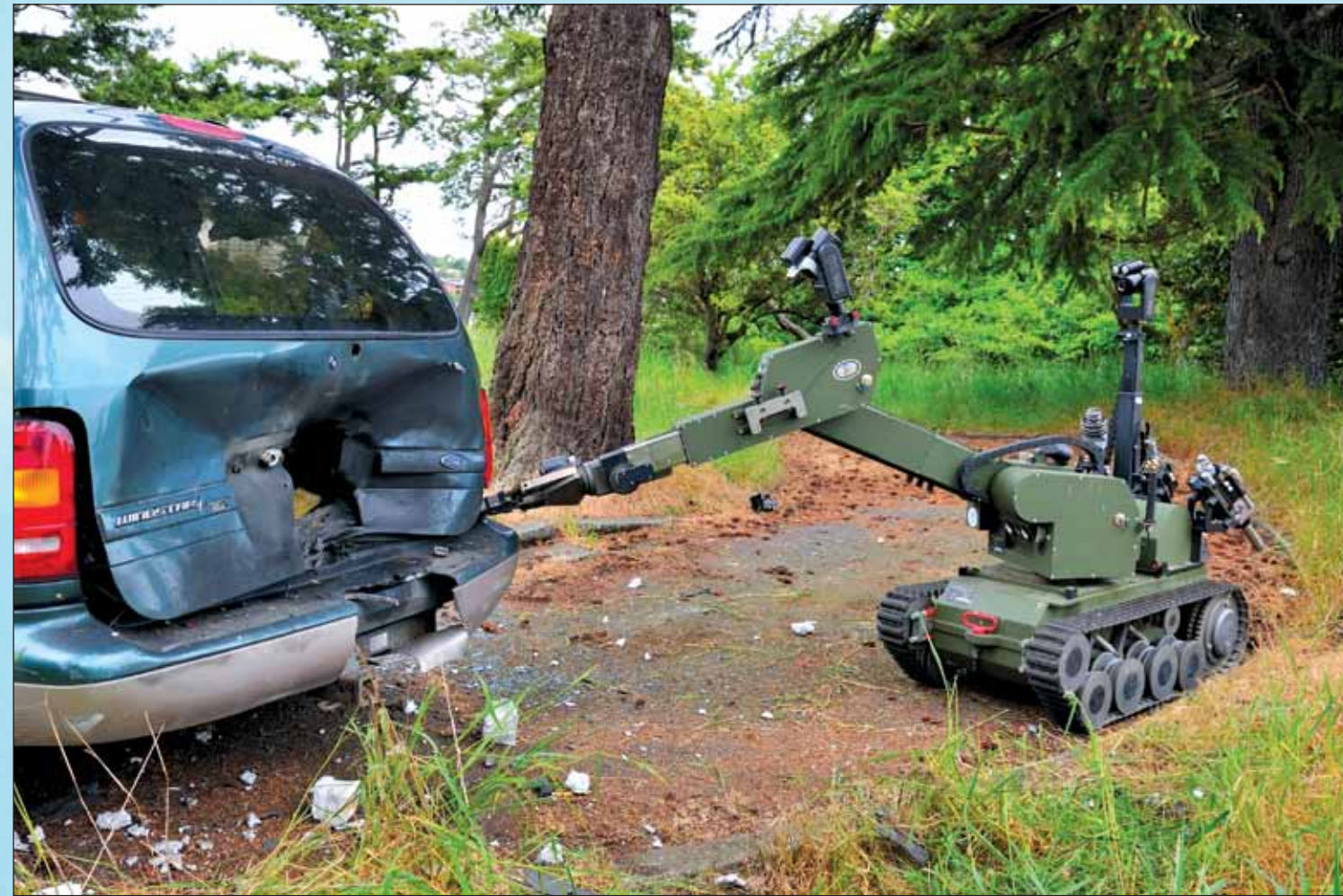
Images by: LS Zachariah Stopa, MARPAC Imaging Services Bomb disposal robot tEODor investigates a simulated improvised explosive device after blowing the door latch.
