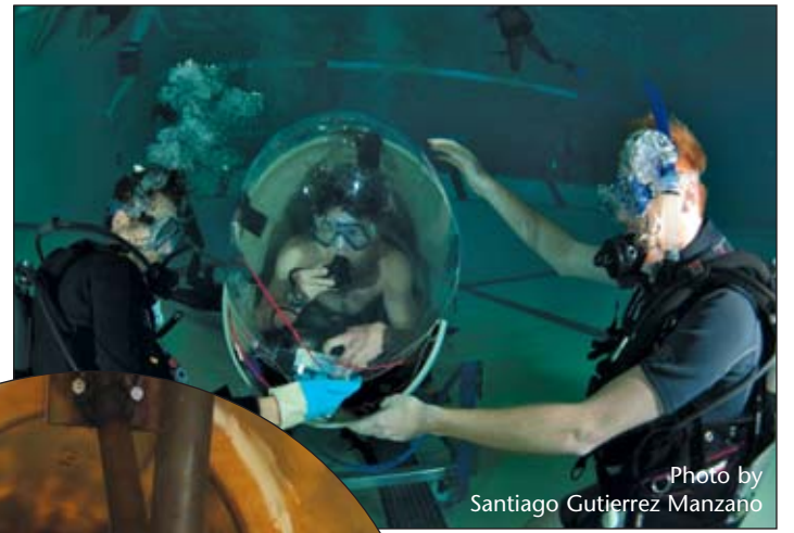
Top: Club members fit the front dome underwater to enclose the pilot in the submarine prior to a test race.
