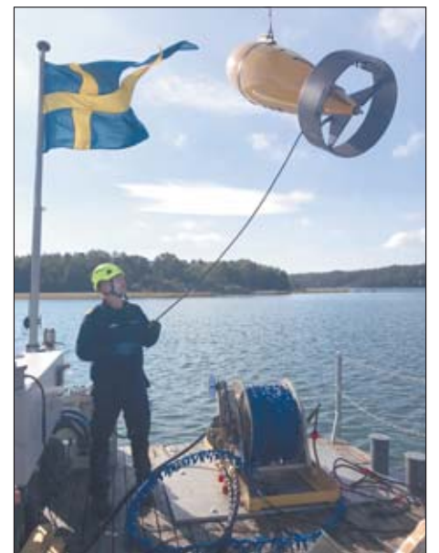
A Canadian sound source is deployed. It simulates the acoustic signature of a passing vessel.
