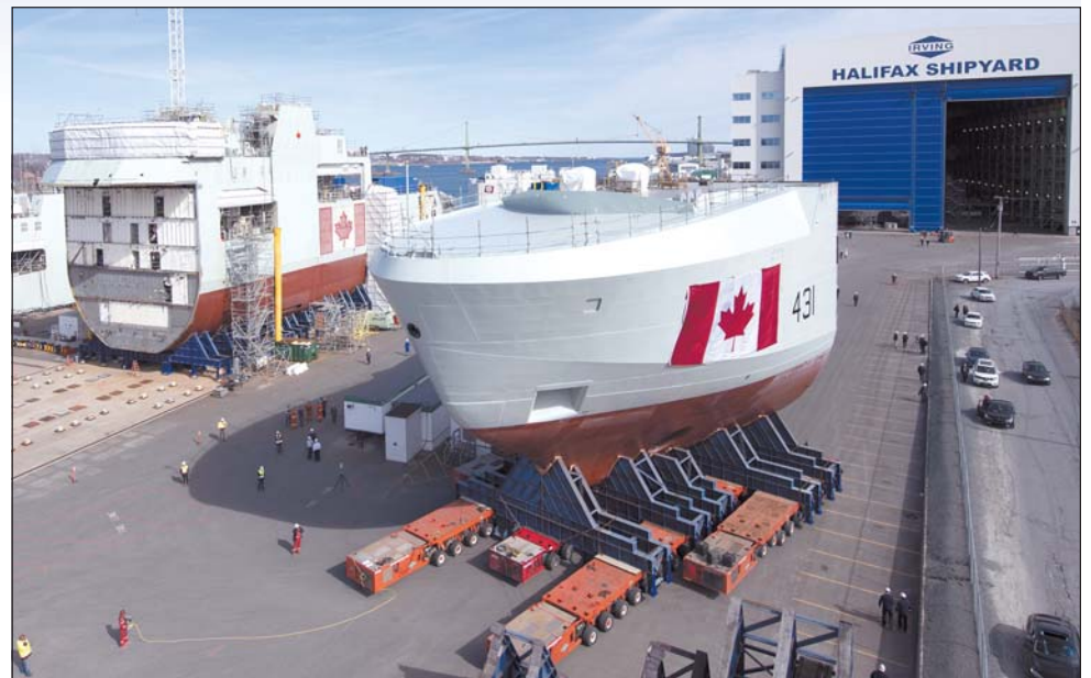
The bow mega block section of the future HMCS Margaret Brooke is moved outside at Irving's Halifax shipyard.
