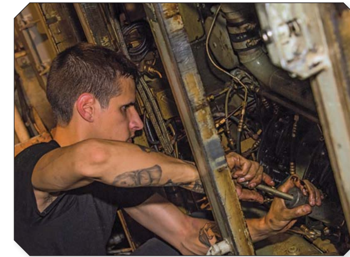
Above: Leading Seaman Dan Zaperty works on one of the ship's diesel generators during Operation Projection in the Pacific Ocean on Aug 5. Left: Leading Seaman Alexis Côté-Lapointe, member of Regina's boarding party, conducts live fire training.
