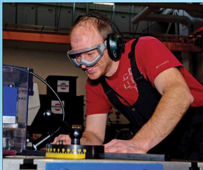
Russel La Rose, a Sheet Metal Fabricator working at the "notcher".
