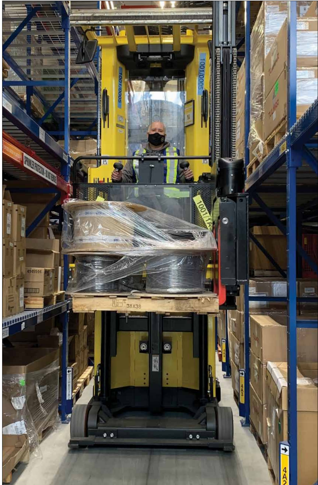
Carlo Legg puts spools of material away into the High Bay racking using one of four narrow aisle wire guided forklifts.
