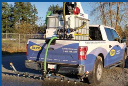
All-In-One Combo Unit STORMSTOP Brine Maker & Brine Sprayer in one package.
