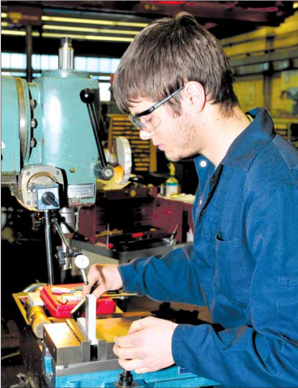
Quinn McCullough, a machinist apprentice at Fleet Maintenance Facility Cape Breton, carefully measures and cuts 90 degree pieces of aluminum for projects around the base.
