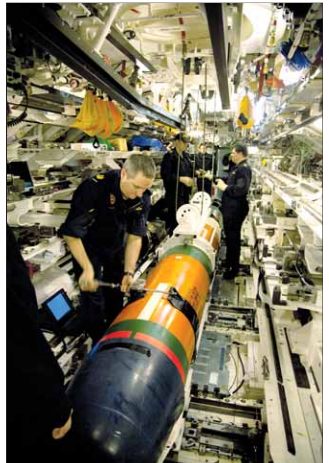
PO2 David Johnston, a senior weapons technician and torpedo instructor, prepares the exercise version of the MK48 Heavyweight Torpedo to be fired from the submarine.
