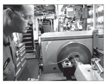
LS Tristan Collier, a Marine Engineering Technician aboard HMCS Calgary, machines a piece of aluminum using the ship's lathe during RIMPAC.
