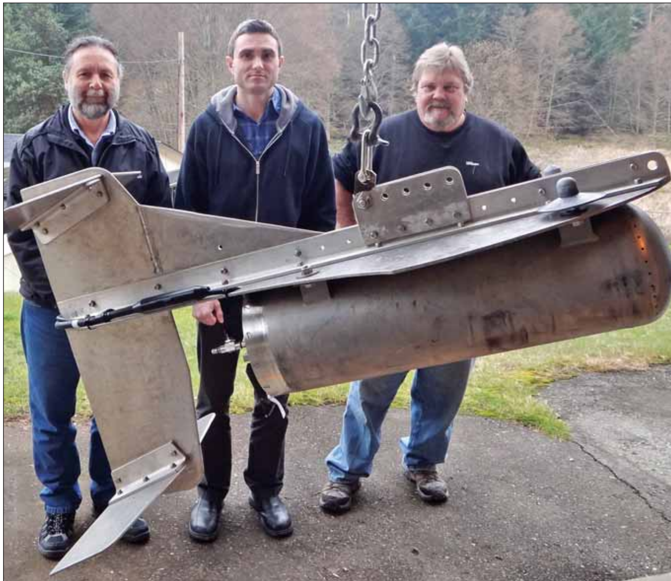
Left to right: Canadian Forces Maritime Experimental Test Ranges employees Bill Cooper, Owen Taylor and Phil Ross with the MR 219 Moving Coil Projector housed under the hand-built tow body.
