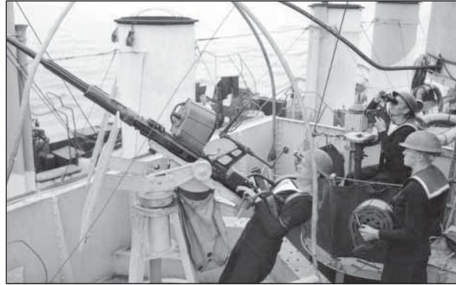
Crew aboard HMCS Morden demonstrate the ship's 20-mm Oerlikon anti-aircraft gun during training off Halifax on Aug. 3, 1943, shortly before sailing to Plymouth, England.
