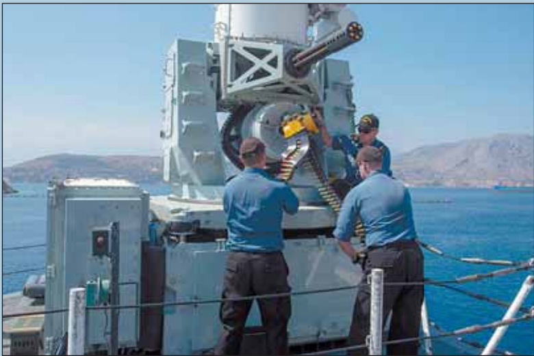
Photos by Cpl Blaine Sewell, Formation Imaging Services Members of the Combat Systems Engineering (CSE) department replace the ammunition in the Close in Weapons System on board HMCS Charlottetown, in Souda Bay, Greece, during Operation Reassurance.
