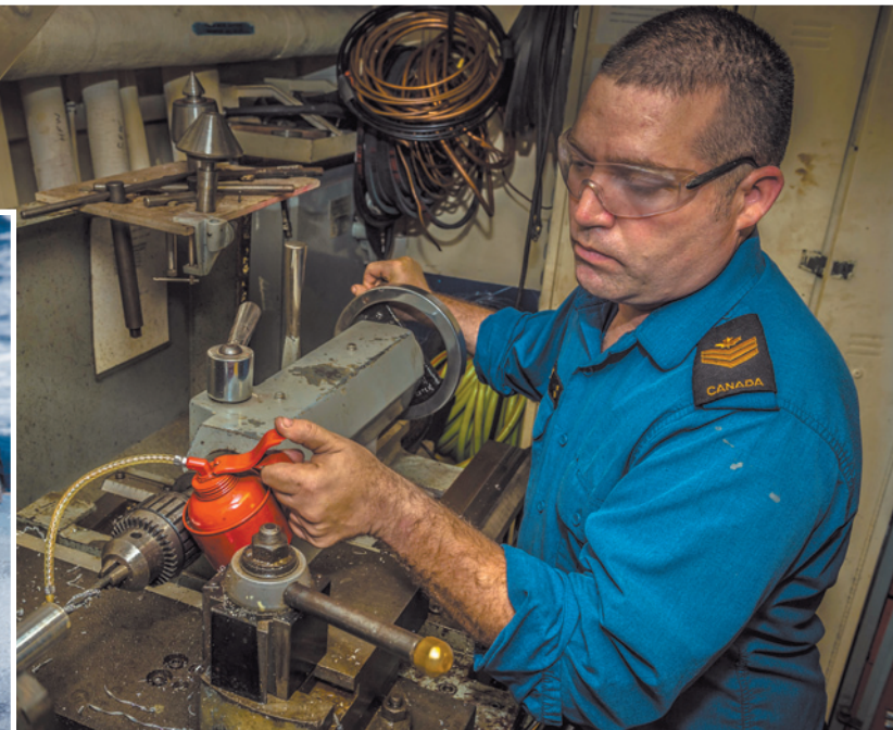
Photo: Tony Chand, Formation Imaging Services Petty Officer Second Class Andrew Childs, a Marine Systems Engineer onboard HMCS Fredericton, machines new parts on the metal lathe during Exercise Spartan Warrior.
