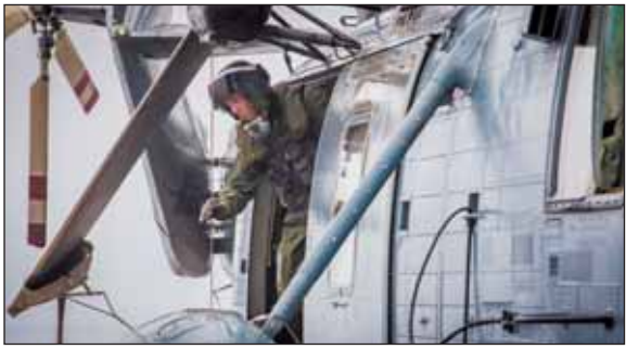
A member from 443 Maritime Helicopter Squadron inspects cables on a Sea King helicopter bound for work up training aboard HMCS Winnipeg.
