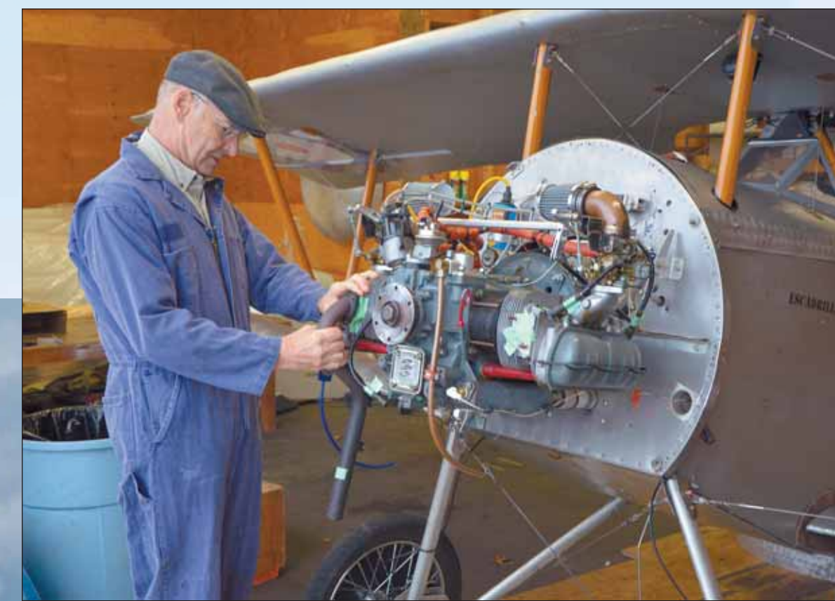
Former Canadian Armed Forces helicopter pilot, Major (Ret'd) Paul O'Reilly tinkers with the Volkswagen engine of his First World War replica of a Nieuport II.
