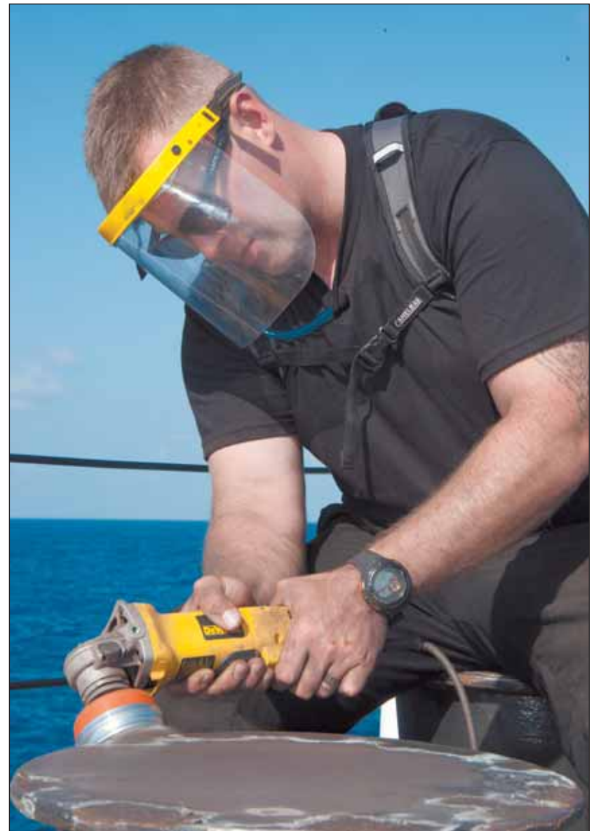
Leading Seaman Chris John prepares the fo'c'sle for painting by sanding off old paint.
