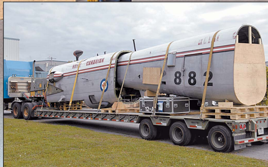
A combined team from the RCAF's Aerospace and Telecommunications Engineering Support Squadron (ATESS) and the National Air Force Museum of Canada dismantle the KB882. It will be restored to its post-war Mark 10 AR (area reconnaissance) configuration with the aid of donations and volunteer efforts. Restoration is expected to take five to seven years.
