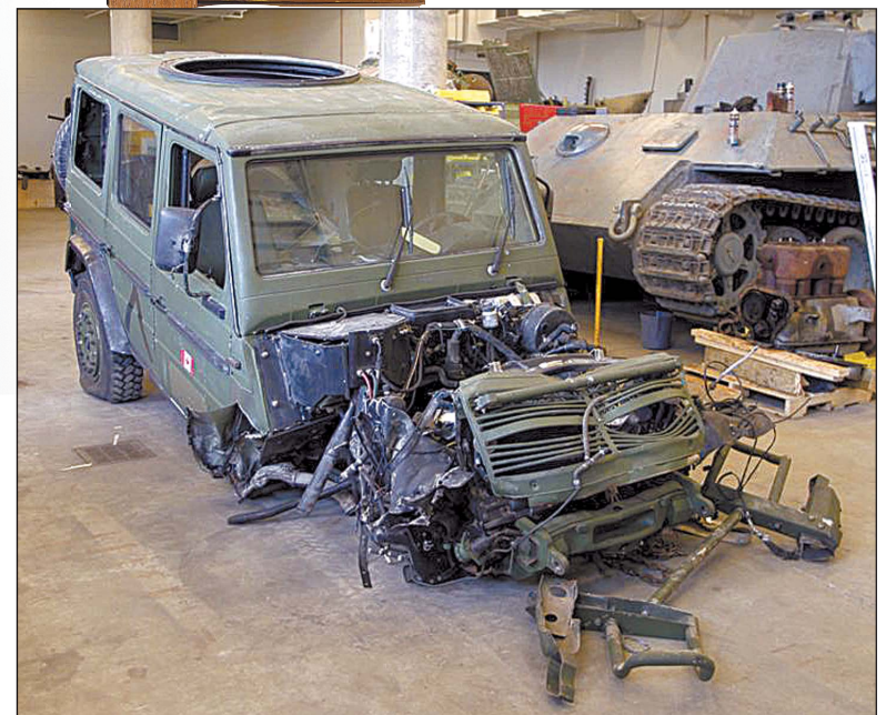
In December 2005, Afghan insurgents detonated an improvised explosive device that destroyed the front of this G-Wagen. Captain Manuel Panchana-Moya, Privates Ryan Crawford and Russell Murdock, and a journalist were saved by the vehicle's protective armour. The blast threw the vehicle's engine nearly seven metres.
