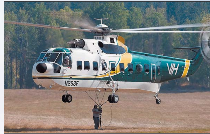
Left: A VIH Sikorski S-61 helicopter, the civilian version of the Sea King, hooks up a long line during a job.
