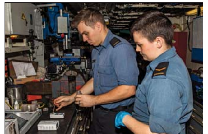
Able Seaman Kendra Wrestling and Ordinary Seaman Sterling Fox measure the coolant quality for the diesel generator during Operation Projection.
