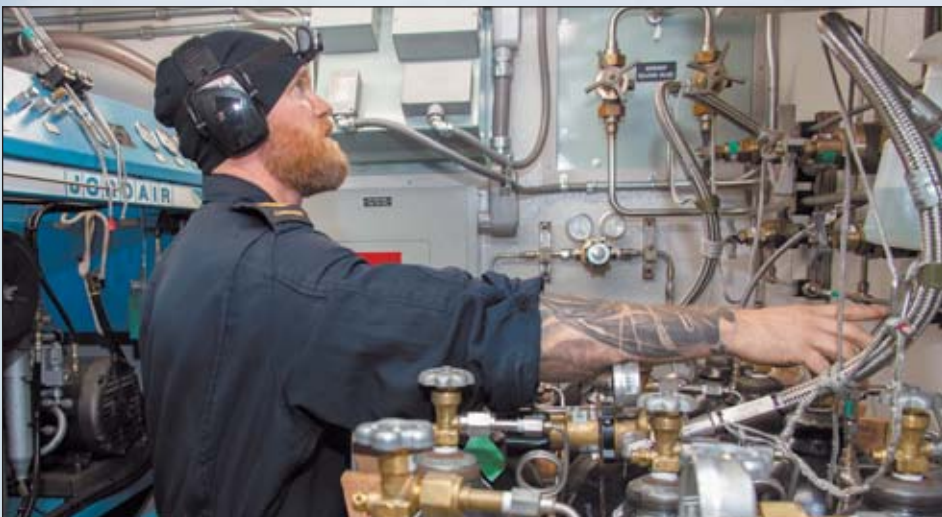
Photo by MCpl Gabrielle DesRochers, Canadian Forces Combat Camera Master Seaman Casey Johnson, Canadian Armed Forces Clearance Diver, conducts flash up procedures on the Containerized Diving System, as part of the pre-dive preparations.
