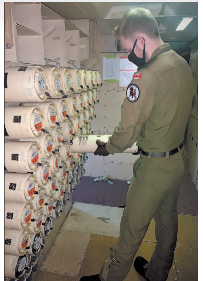
Right: An Airborne Electronic Sensor Operator with 407 Long Range Patrol Squadron takes an inventory of sonobuoys used to detect underwater sounds on board a CP-140 Aurora during Exercise Sea Dragon, held at Andersen Air Base, Guam. Photo Major Mathieu Kuhn
