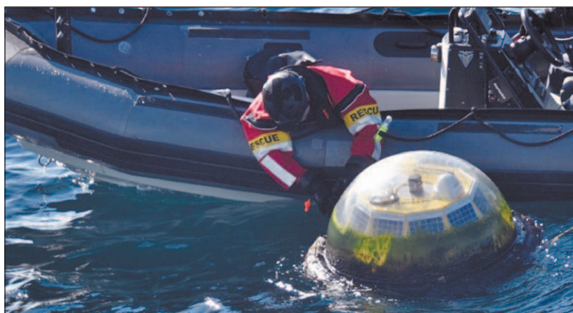
A bridle is attached to the buoy so the ship's crane can safely lift it on board.
