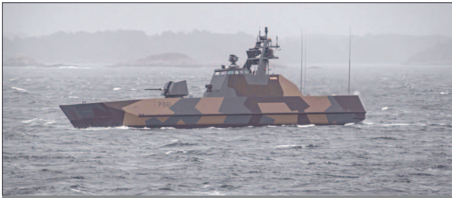
Royal Norwegian Navy Corvette HNoMS Storm participates in the NATO Maritime Command Exercise Dynamic Guard 21-1 off the Norwegian coast. This Skjold-class Corvette is a large, superfast, stealth missile corvette that specializes in littoral warfare. Capable of 60 knots, it is one of the fastest warships in the world.
