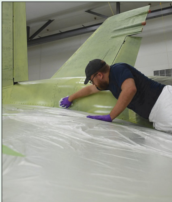
Corporal Martin Savard, an aircraft structures technician, cleans off the surface of a fighter jet before the first layer of NATO standard grey is applied.
