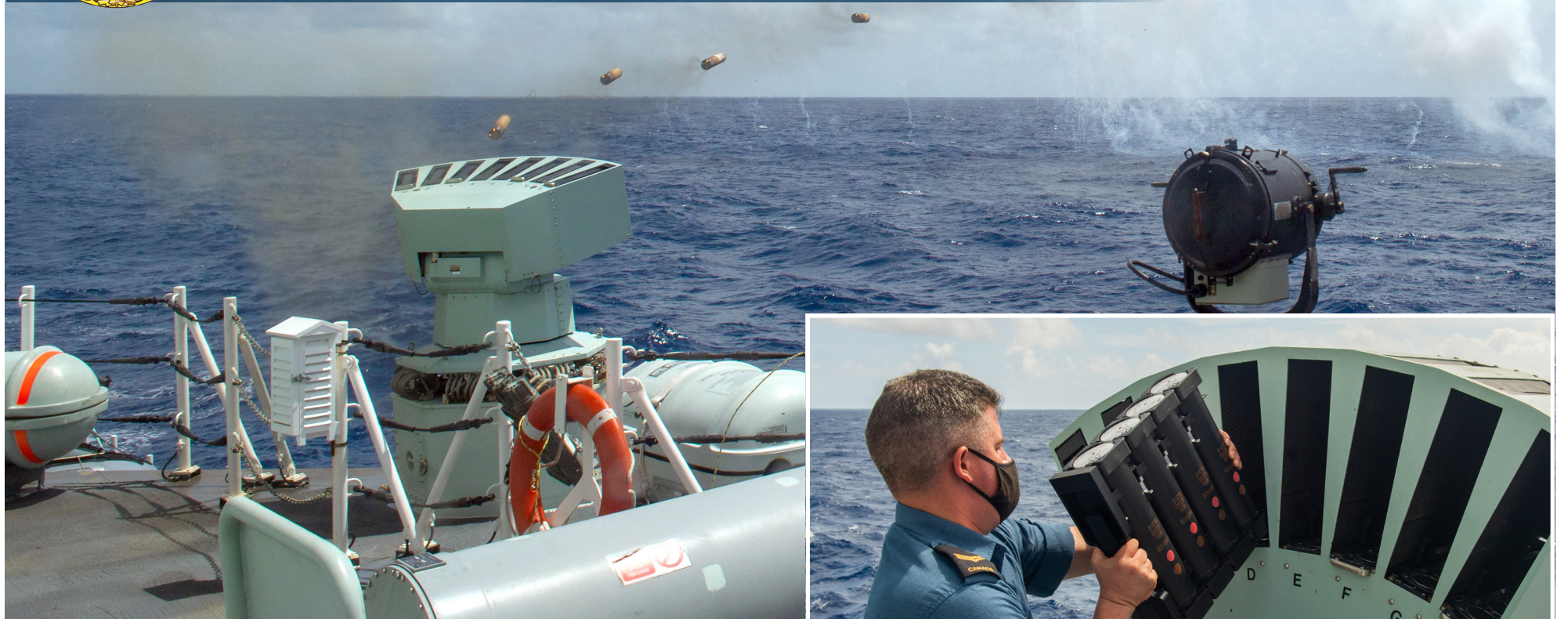
HMCS Vancouver (FFH 331) fires the multi ammunition soft-kill system (MASS) from the bridge during Rim of the Pacific (RIMPAC) 2022. Photos: Sergeant Ghislain Cotton
