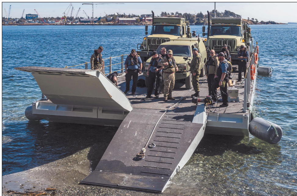
Canadian sailors train in Esquimalt, B.C., using the new sea-to-shore connector, a modular, self-propelled barge designed to support the future Joint Support Ships.
