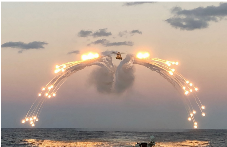
Canuck, Vancouver's embarked CH-148 Cyclone helicopter, practises a flare jettison, which seeks to confuse heat seeking missiles, while in the Philippine Sea.
