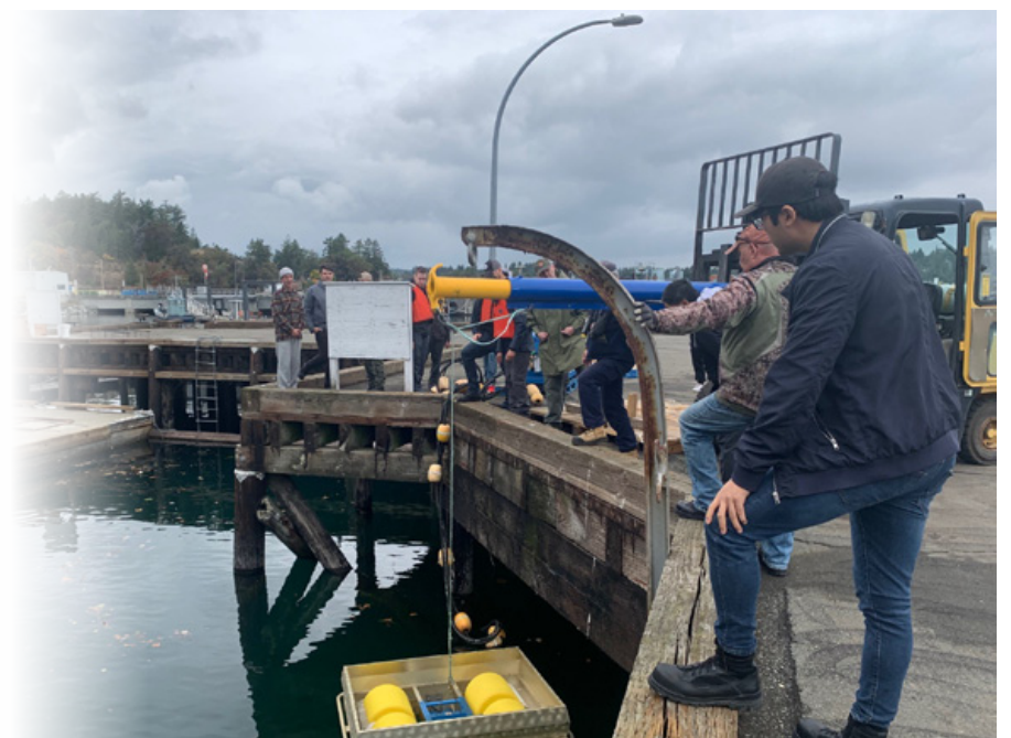
An oleophilic drum skimmer is laid in water as the participants engage in an oil spill scenario during the Marine Spill Response course.
